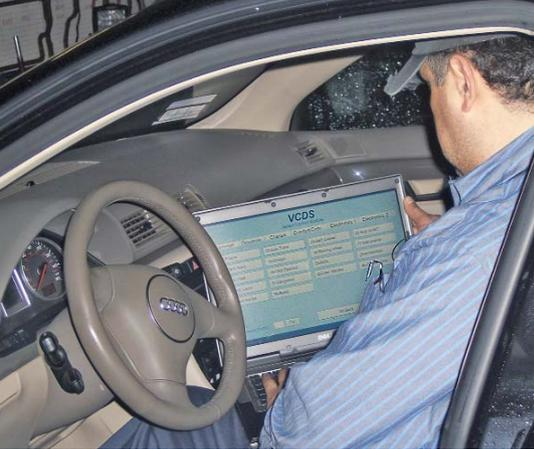
**Octavio is running a diagnostic procedure on an Audi.**
